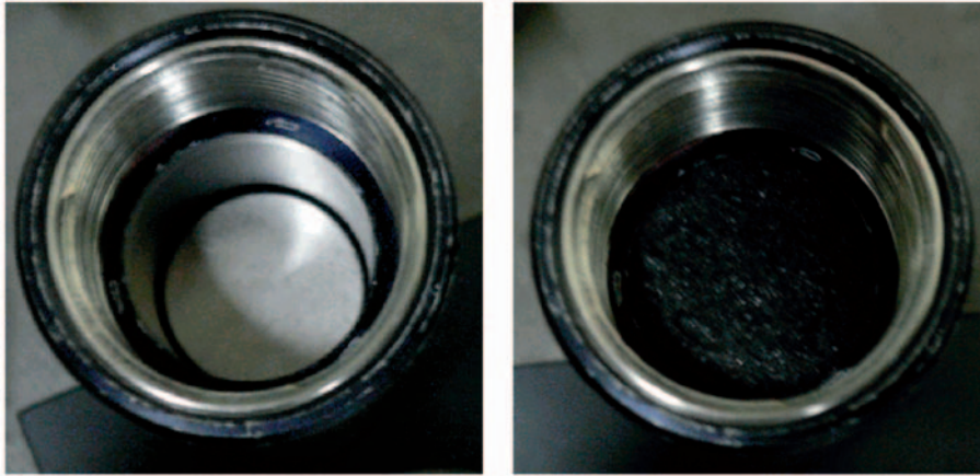
Figure 5. Tube with the magnet and with the magnet and a sample of MR foam.
